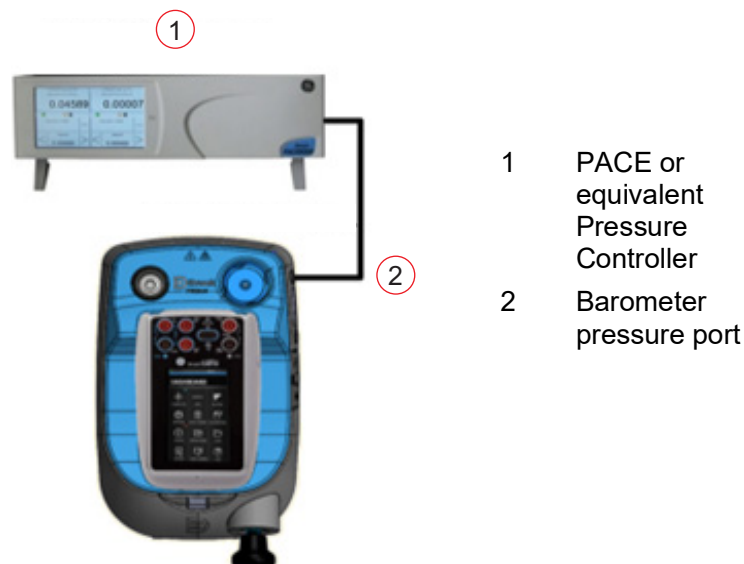
Figure 4-6: Barometer Calibration Setup
