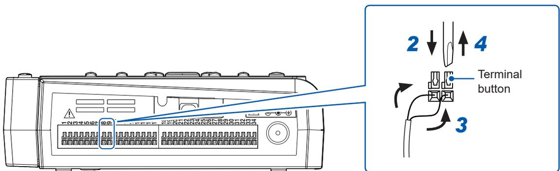
Example connecting to pulse 4 and GND
