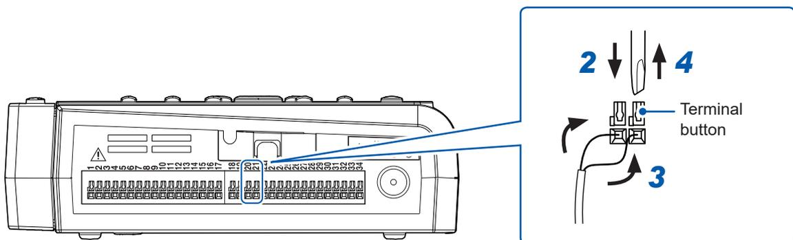
Example connecting to external input 2 and GND
