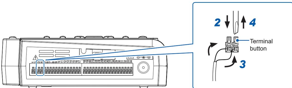
Example connecting to voltage output 2 and GND
