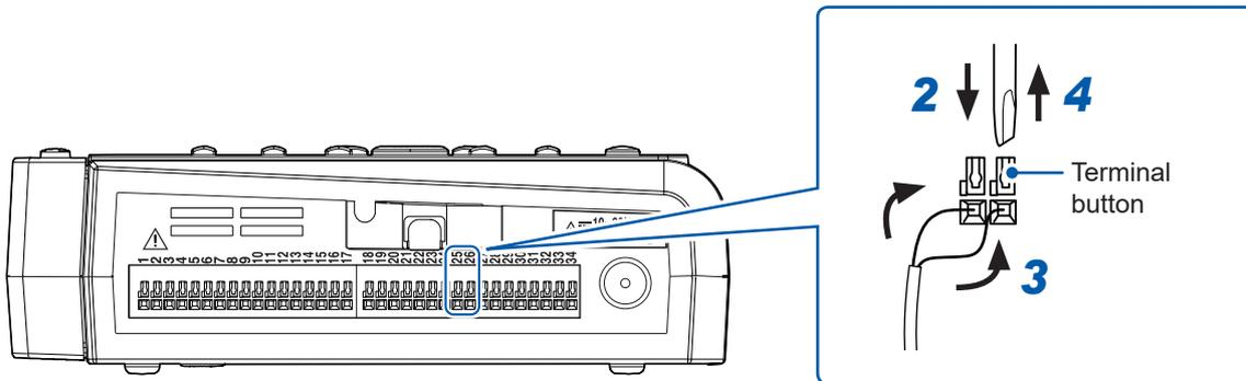
Example connecting to alarm output 4 and GND
