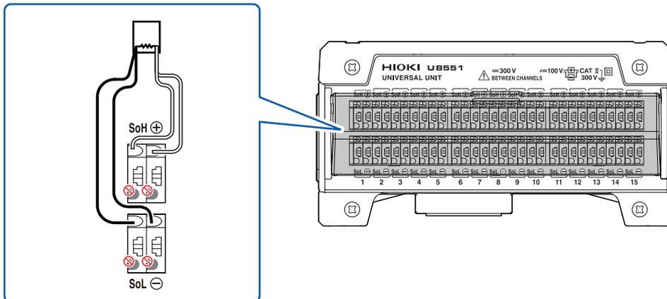
Connect the resistor using a 4-wire setup (the instrument cannot measure 2- or 3-wire setups).
