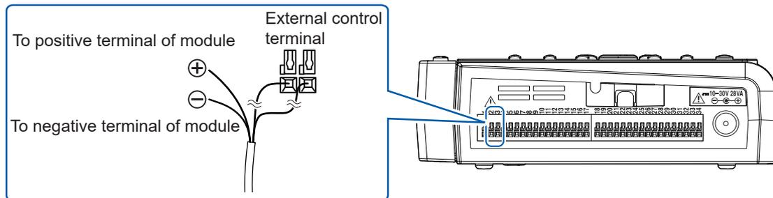
To supply power to the Z2000, set Voltage output terminals 1 or 2 to **[12 V]**. See "8.1 Configuring Voltage Output (VOUTPUT)" in the Instruction Manual.
