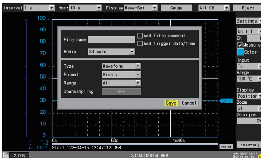
The instrument can load binary-form (LR8450-specific-form) waveform data only. When you do not name files, the instrument will automatically name them.
