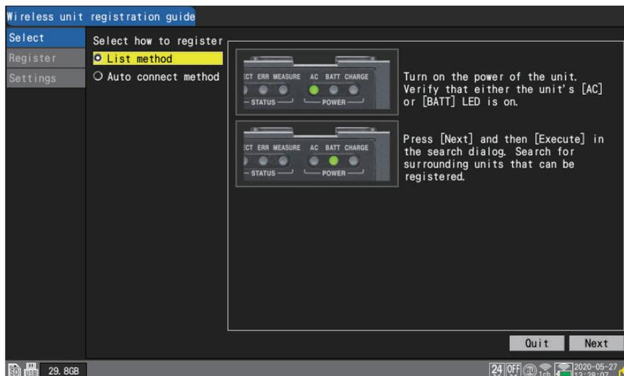
Once the registration completes, the wireless module's **CONNECT** LED will light up.
