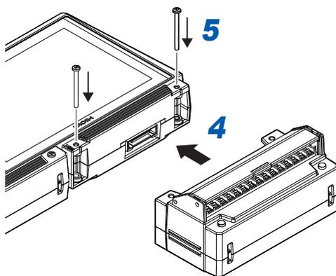
**4** Connect the plug-in module to the connector on the instrument.
