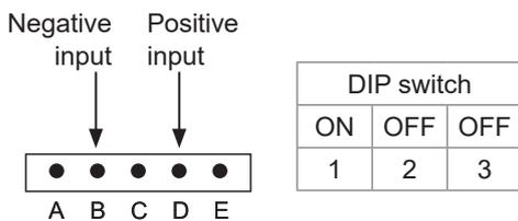
When connecting a converter, the terminals function as indicated below. If the converter output utilizes a connector (such as NDIS connector), use a cable with a connector on one end and loose wires on the other to make the connection.
