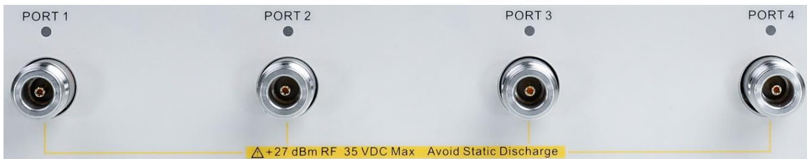
Figure 5-6 Front panel RF connectors (4-port VNA)
