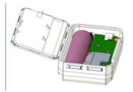
Remove the circuit board and battery (red arrow) and dispose of them separately in accordance with local regulations.
