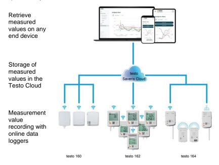
If limit values are exceeded, you can be alerted directly via push notification of limit value violations thanks to the testo Smart App. Alternatively, you can be notified by email or SMS.
